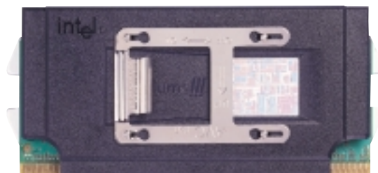
Example of an incorrectly installed retention clip
