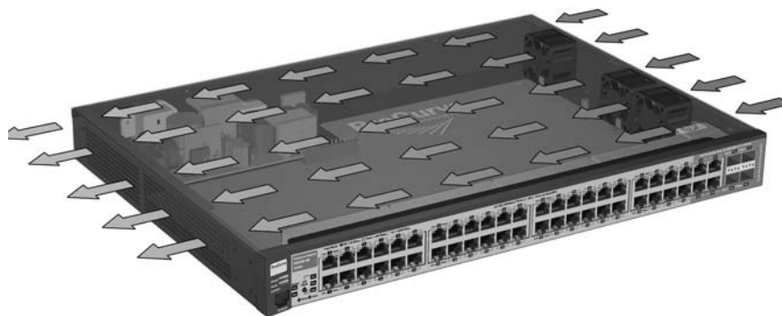
Figure 2-1. Air flow direction of the 2510G switch
