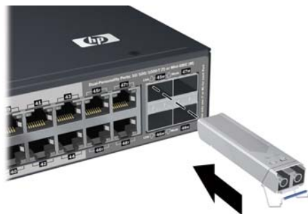
Figure 2-2. Example of installing a mini-GBIC (SFP)
