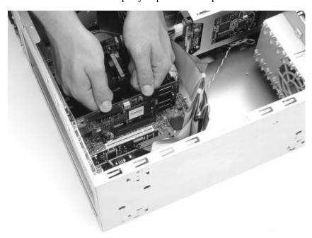
5. Once you are certain your Stealth II G460 is installed properly in its slot, secure to the computer frame with the screw you removed in step 2.
