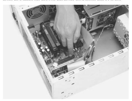
2. Remove the screw attached to the bracket cover and remove the bracket plate.
