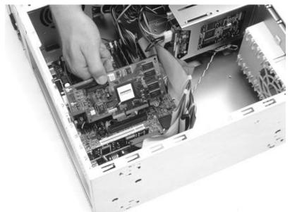
Make sure the VGA connector end of the card is facing the open end of the bracket you just removed.
