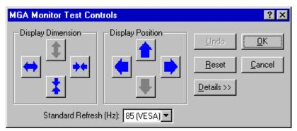
**Display Dimension** – Use these controls to expand or shrink the display horizontally or vertically.
