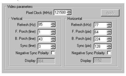
When you click the **Details** button, a **Video parameters** panel is added to the **MGA Monitor Test Controls** dialog box. This panel displays the video timings for the current mode, and dynamically shows changes in parameter values when you use the **Display Dimension**, **Display Position** and **Standard Refresh** controls.
