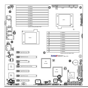
A. VGA Enable (X8DAH+-F/(-LR) only) B. 1394a 1/2 Enable
