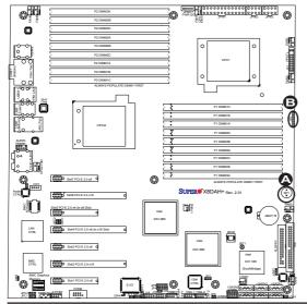
A. Internal Speaker (Buzzer)B. PWR LED/Speaker
