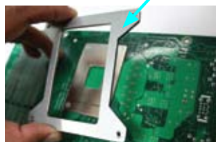
Install the Heatsink Bracket on the reverse side of the board.
